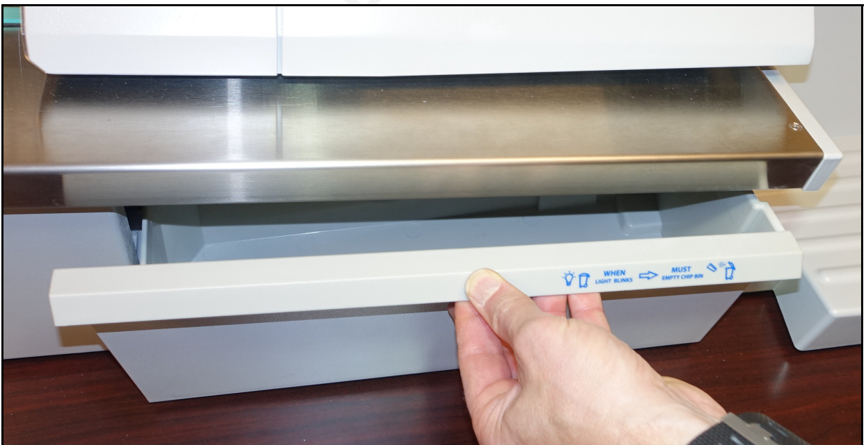
Figure 2-10: Bin tray removal interlock triggering
