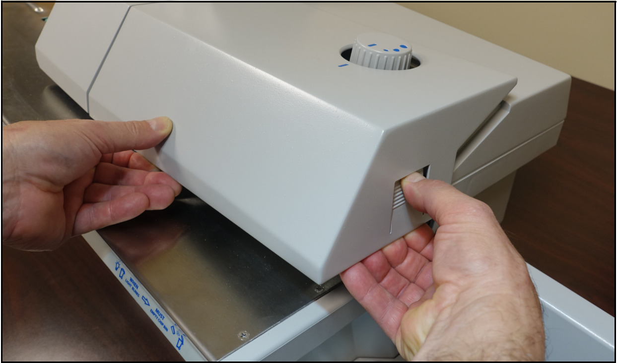
Figure 2-9: Top cover removal interlock triggering
